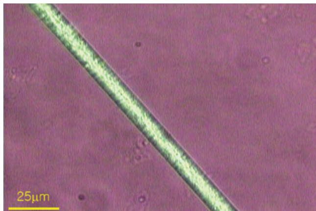
Figure 1 Picture of a fiber of CN-PPTA/3 wt % clay layered silicate observed through the polarized optical microscope under a cross polarizing filter. [Color figure can be viewed in the online issue, which is available at www.interscience.wiley.com .]
